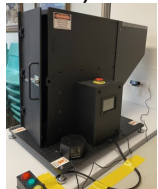
Figure 1- Test box with dark sides and clear front pushed up against a wall with a camera to allow for real-time remote viewing
